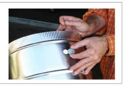
2. Holding the blade in position, pass the 3/8" square bar through the bushings and channel in the blade.
